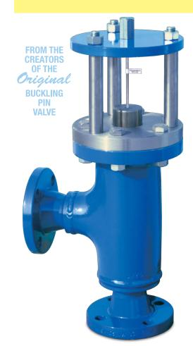
The **Model C** holds a bubble-tight, closed position until pressure reaches an exact set point. At set point, the valve instantly opens to relieve pressure from a protected system.
