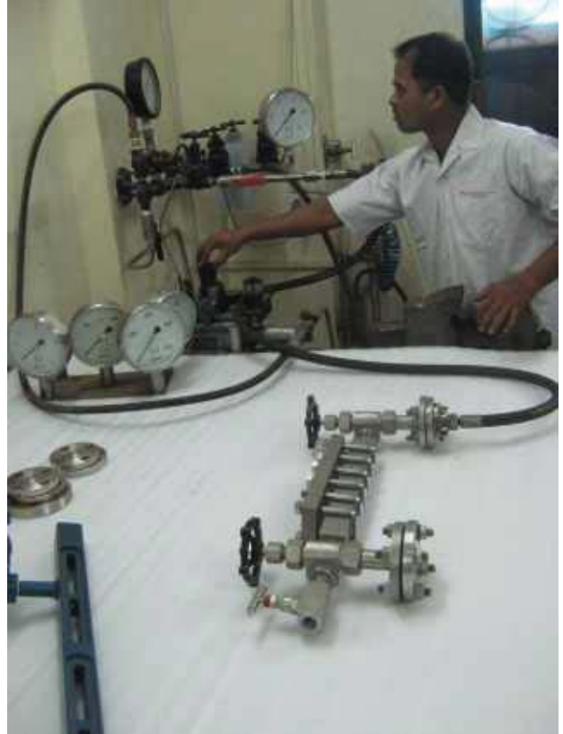
Hydro test bench and calibration test bench applicable with helium leak test for gauges for perfect tight sealing feature
