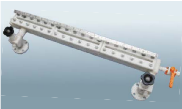
Reflex level gauge at 150# rating at 125 deg cent and FF end connection with auto ball check valve and drain valves in Polypropylene material
