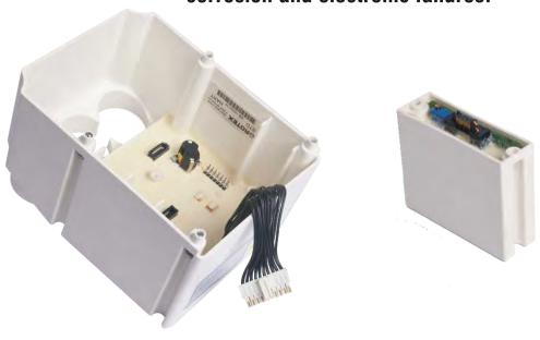
Major failures are seen in electronics mainly due to moist instrument air or external humidity, damaging the exposed electronic parts.
