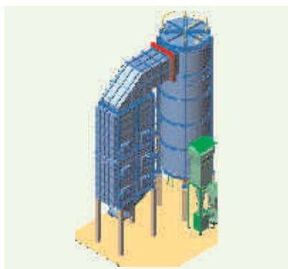
Vertical up fired OTSG for Bitumen firing at JACOS site in Canada
