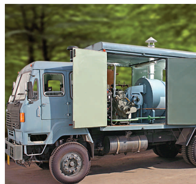
Trailer mounted mobile steam generator.
