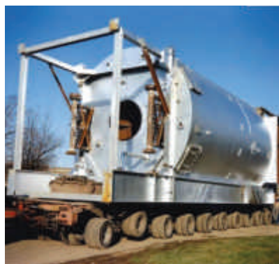
45 Te/h Coil Boiler being transported
