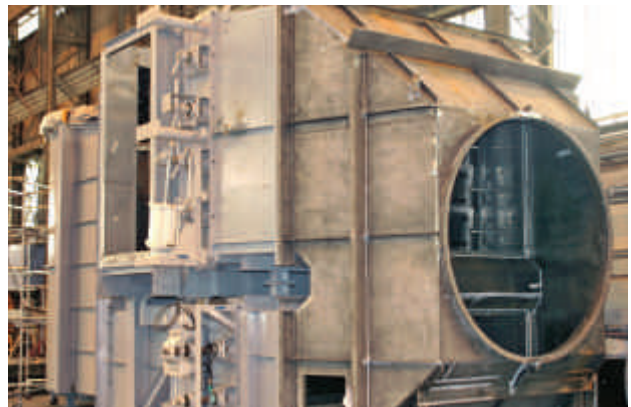
Trial assembly of inlet/outlet boxes of a WHRU
